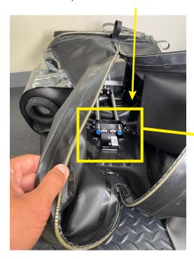
The plate mounts **directly** to bottom of ARRI Mini or Mini LF with standard 4 hole pattern.
