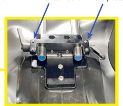
HydroFlex optional plate shown at left is equivalent to ARRI MAP-2 plate:
