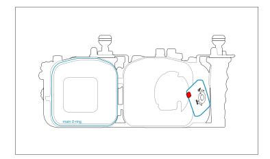
before closing the housing, clean and lubricate the main O-ring
