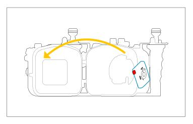
flip open the back housing when lock latch is aligned to 'open' position
