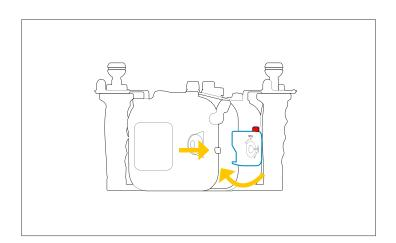
insert the housing shaft into the shaft hole and then rotate the lock latch clockwise until you hear and feel it click into place
