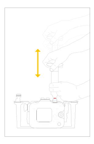
connect hand pump to the valve and pump several times until it reaches the target vacuum level
