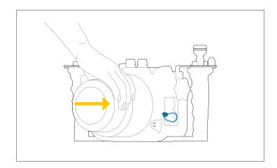
lubricant the port O-ring before mounting
