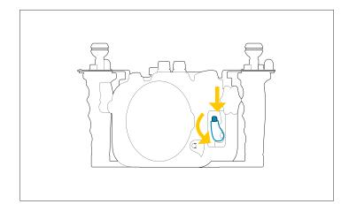
depress port lock safety button and rotate anti-clockwise
