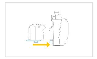
slide the camera tray back into the housing along the tray rail
