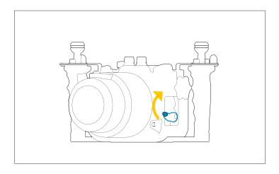
rotate locking lever clockwise to lock
