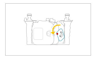
turn housing lock latch anti-clockwise to open the housing
