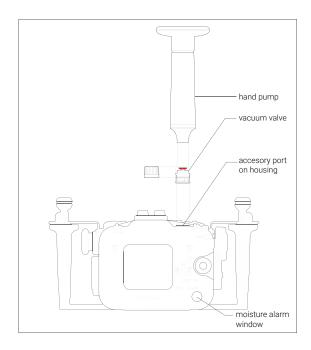
remove the plug of M14 accessory port from the housing
