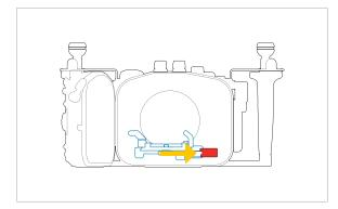
unlock camera tray lever and remove the tray from the housing
