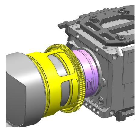
Install RF mount lens to camera, and Lock the RF mount Locking ring. For use with EF lens, Canon EF –
