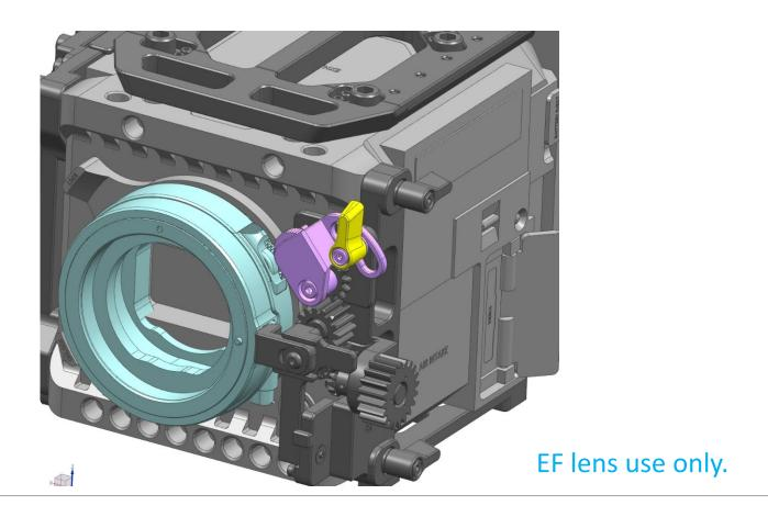
• As for use with Control Ring/V-ND mount adapter, please adjust the control dial position as shown above.
