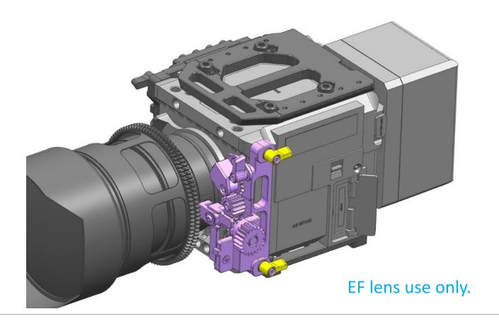
• Install the EF REL Block for use with EF lens and EF–RF Mount adapter, Fasten it with two thumb screws.
