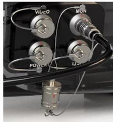
When connecting or disconnecting the cables **grip the connector bodies**. Do **not** pull on the cables, as this will damage the connector assembly
