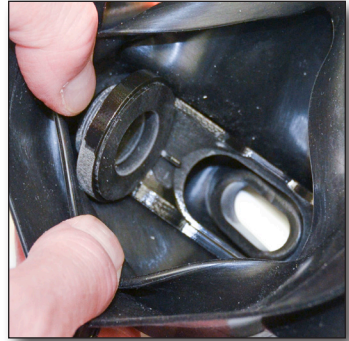
Figure 11: Inner Frame Removal
