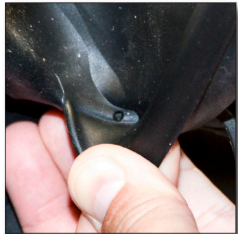
Figure 4: Visor Drain Hole
